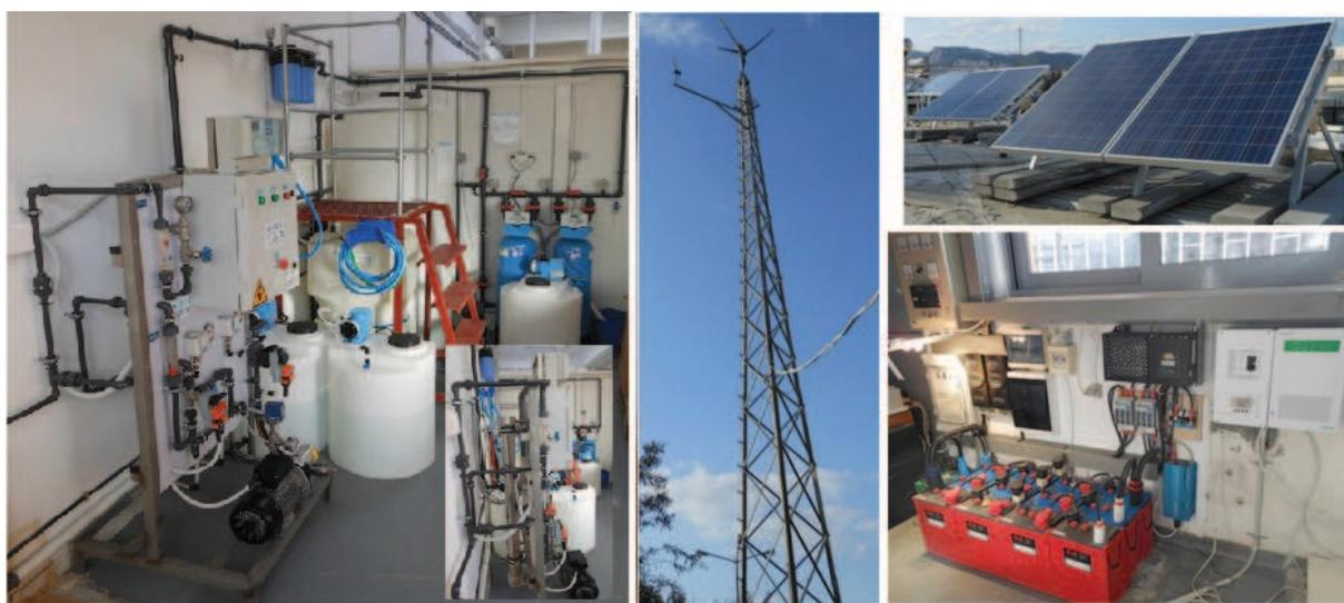
Fig. 2. SEALAB RES hybrid (including desalination) experimental unit
